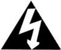
The lightning flash with an arrowhead of an equilateral triangle is intended to alert the user to the presence of dangerous voltages within the products enclosure. If not careful, these voltages are of sufficient magnitude to constitute an electric shock to persons.
